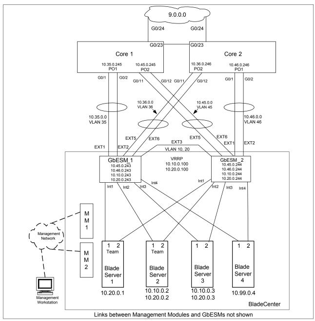
Figure 7-7 Layer 3 Sample Configuration (Dynamic routing)
